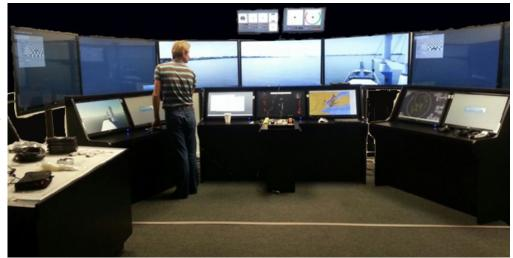
ECDIS stands for Electronic Chart Display and Information System and is a computer-based navigation system that complies with all IMO regulations and can be used as the primary alternative to paper navigation charts.
